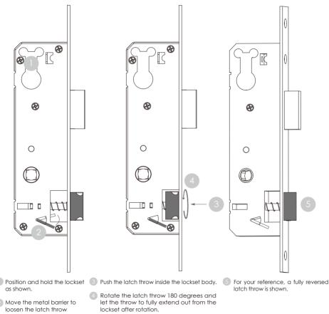
NOTE: If you're installing a Slide Edition skip this step and proceed to Step 3. If you're installing a Multi-Point Lockset for a Swing Edition, see next page to adjust the latch throw. FOR MULTI-POINT LOCKSET MODELS: PGMB138H 1 3/8" (35mm) / PGMB158H 1 5/8" (40mm) / PGMB134H 1 3/4" (45mm)
