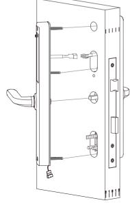
Plug the connection cable of the exterior panel to cable of the interior panel. Once connected insert cable to the door frame holes.
