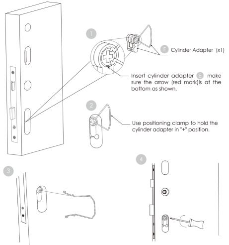
Once adapter is secured, remove positioning clamp by pressing on both sides.
