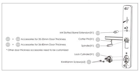
Before installing the key cylinder, make sure your door handle have been adjusted to your door opening direction, see Step 2.
