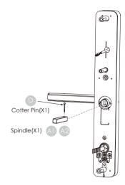
Before installing the key cylinder, make sure your door handle have been adjusted to your door opening direction, see Step 2.
