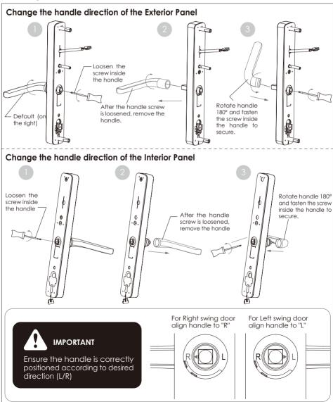
Make sure your door is prepared for installation. If you need to drill new holes, please use the supplied template for drilling holes. Before installing the Lockset (5), confirm the door opening direction (Step 1) and ensure latch throw inclined part is positioned opposite to the opening direction.
