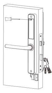
2. Check the lock functions according to user manual after installing the batteries. Use the battery cover to secure the battery compartment and fasten with screw. Congratulations! You have completed the Lockly Guard physical lock installation. To complete your setup, download the LocklyPro app from the iOS or Google Play app Store and follow on-screen instructions.
