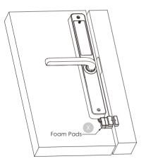
The arrows must be aligned or as closed as possible (less than 3/4"). If IMPORTANT: needed, adjust the position of the sensor magnet using provided foam pads to ensure the Lockly logo blinks red when door opens or closes.
