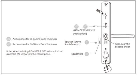
Install the exterior panel onto door. Ensure the spindle, lock cylinder, positioning rods and cable are inserted on the correct holes and passed through the llockset.
