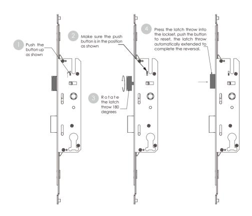
The diagram below shows how to shift the door handle from right to left direction. The default setting of the handle is for right handed door. You do not need to change direction if you have a right handed door.
