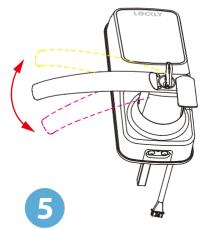
Check that your handle works smoothly by moving it in both the up and down direction.
