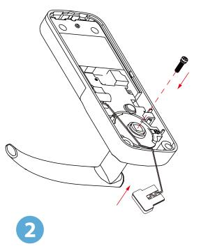
Remove the handle retaining screw and detach the handle. Rotate it to 180° then return as shown.
