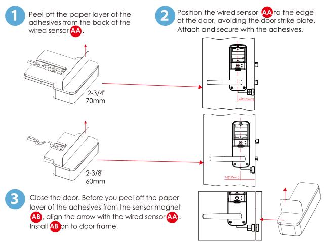
The arrows must be aligned or as closed as possible (less than 3/4"). If needed, NOTE: adjust the position of the sensor magnet using provided foam pads to ensure the Lockly logo blinks red when door opens or closes. Congratulations! You have completed the Lockly Duo<sup>™</sup> physical lock installation. To complete your setup, download the Lockly app from the iOS or Google Play Store and follow on-screen instructions.
