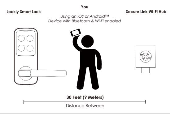
**TIP:** The Secure Link requires a strong wireless signal for optimal performance. Make sure the Secure Link will be installed in a location with a strong 2.4 Ghz wireless signal. Sometimes distances between Wi-Fi hub and lock can vary due to circumstances. If you are having difficulty setting up optimal range of 30/ft or less, we're here to help. Call our customer care team: (669) 500 8835, or visit Lockly.com/help for suggestions and troubleshooting tips.
