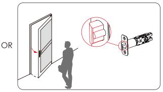
Install deadbolt **()** (top) and latchbolt **()** (bottom) to door and secure with screws **()**. Retract deadbolt and make sure bore hole is horizontally positioned.
