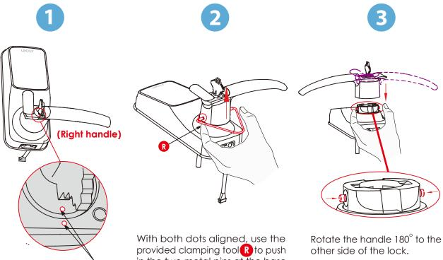
Insert key and rotate lock face so that the two white dots align as shown.
