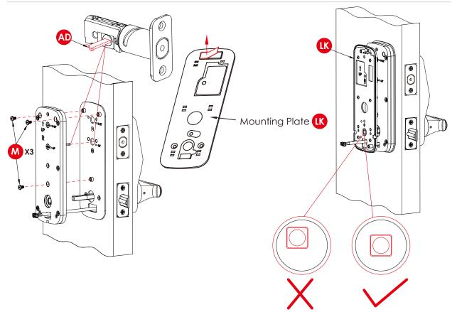
Install plate P onto door. Ensure the torque blade AD is inserted horizontally to the deadbolt. The spindle must pass through the plate. Secure the plate with screws M.
