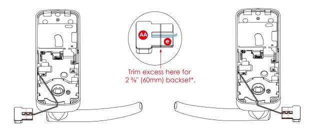
\*Backset - measure the distance of the door edge to the center of the door hole.
