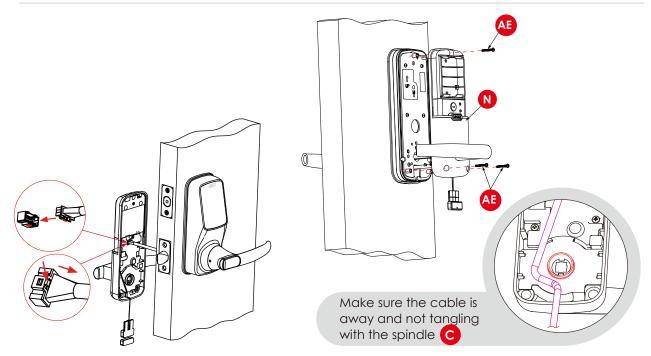
Plug the cable into the interior side of the lock making sure you match the orientation of the plug by matching the red side on the plug with the red side on the lock. Secure the connection by ensuring that the connector is snapped in and inserted tightly.
